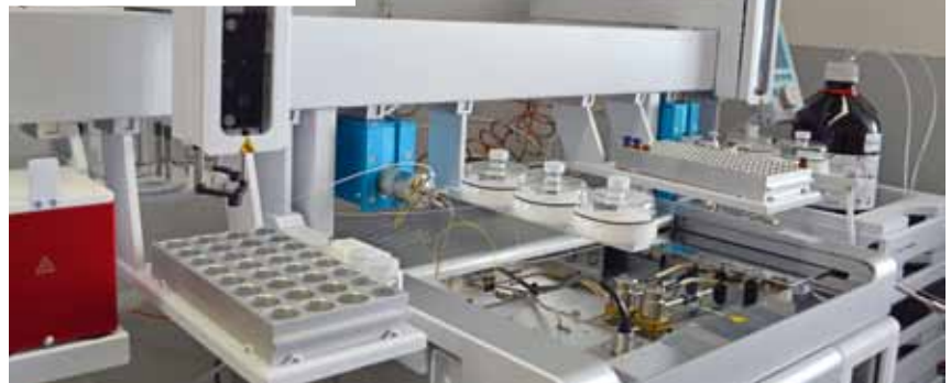
Online coupling of Liquid Chromatography with Gas Chromatography and Flame Ionization Detector for the quantification of the sum of MOSH and MOAH (Instrument from Axel Semrau Company, Sprockhoevel/Germany)
