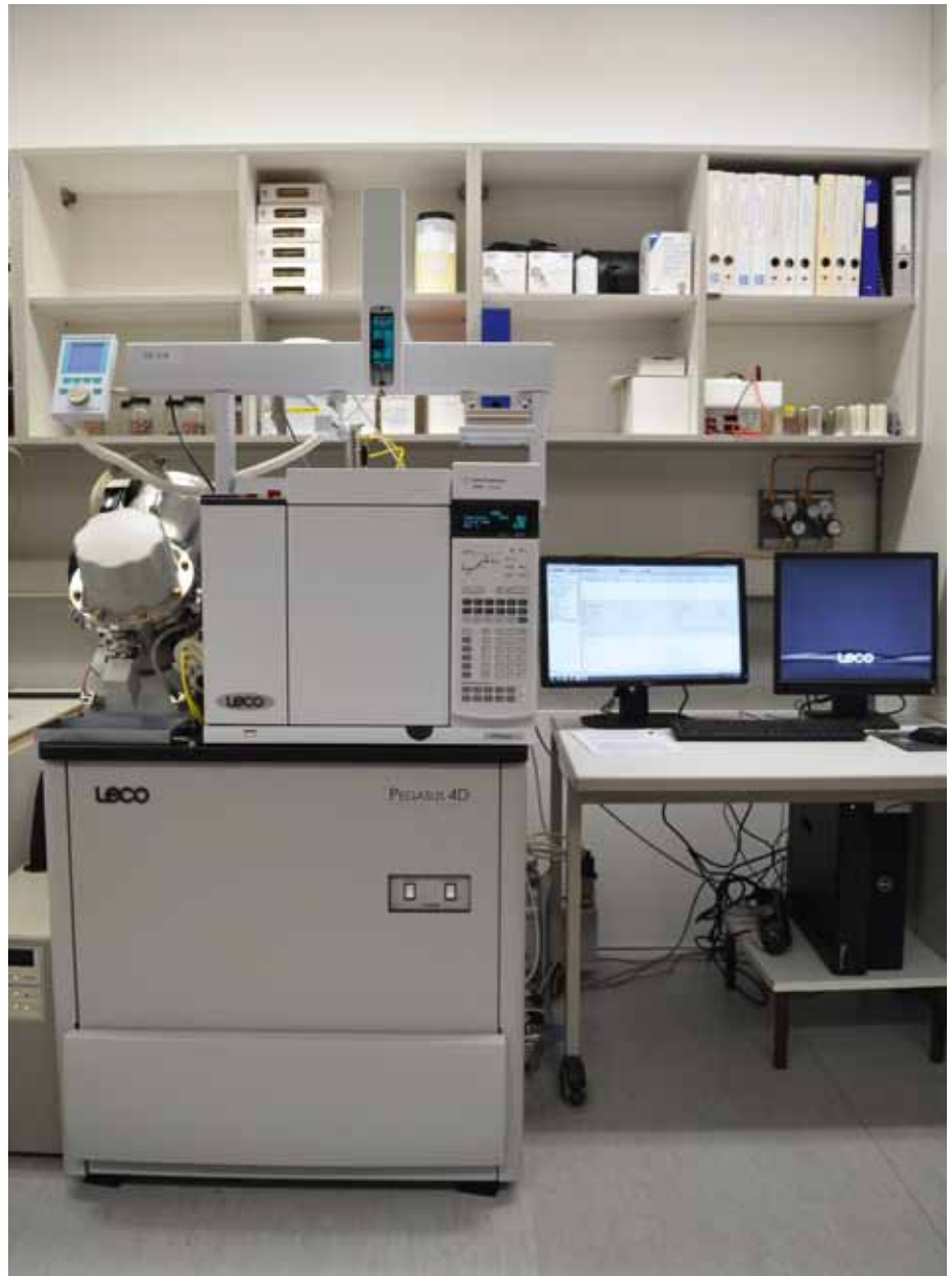
GCxGC-TOF-MS: Comprehensive Gas Chromatography coupled with Time-Of-Flight Mass Spectrometry for the characterization/identification of substances/substance classes (Instrument from Leco Corporation, St. Joseph, Michigan/USA)
