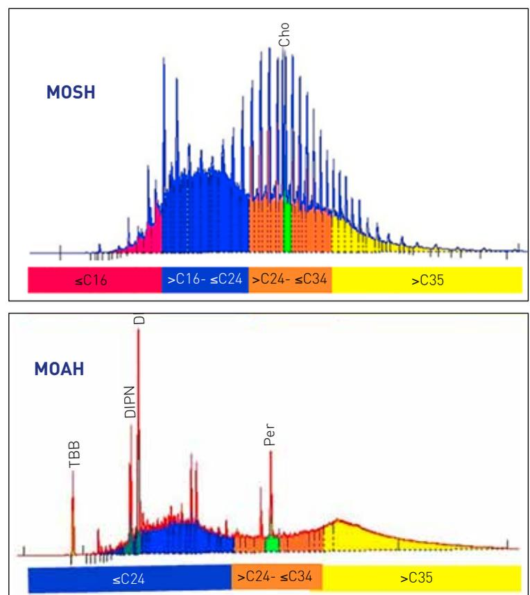
Fig.2 Diagram illustrating the chromatographic “humps”
